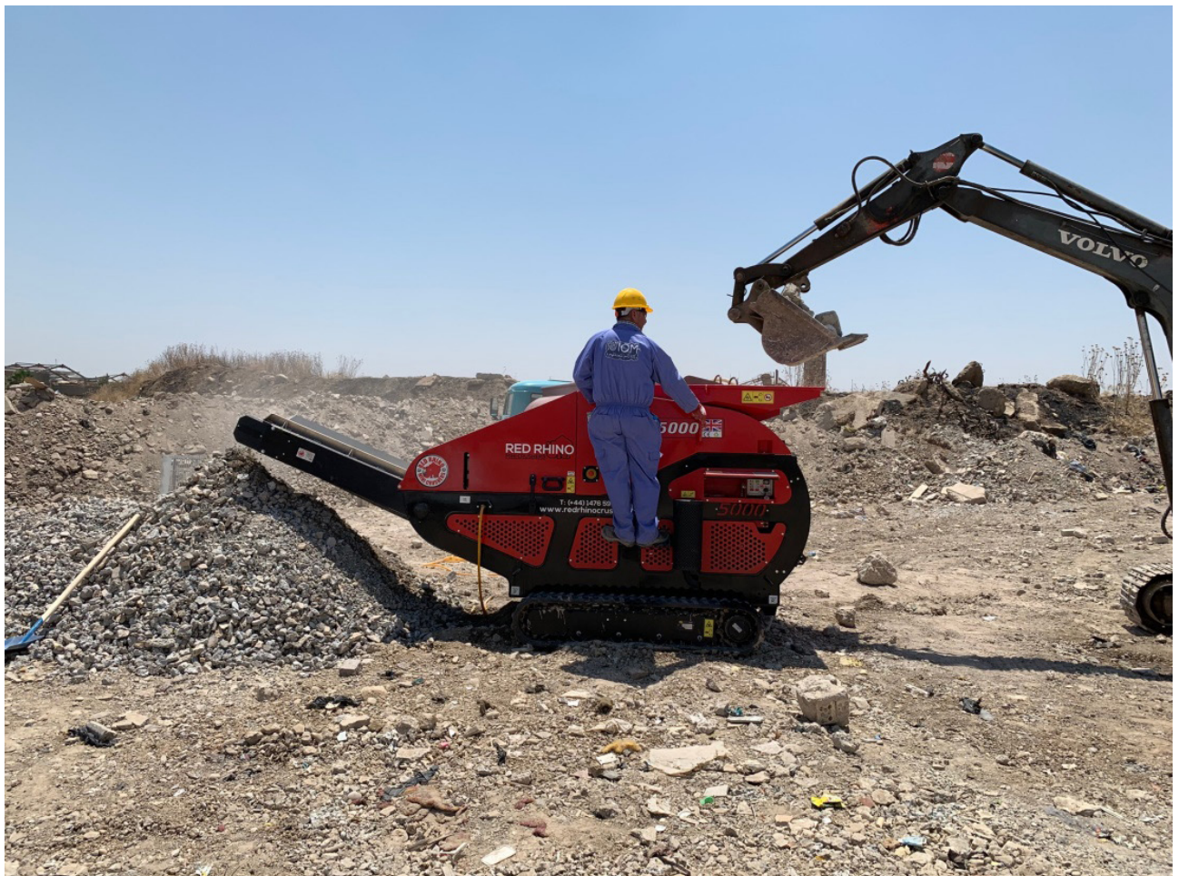
:Small scale crushing of debris by the International Organization for Migration (IOM) at the Mazen Debris Recycling Pilot Site in Mosul ©2020 United Nations Environment Programme
